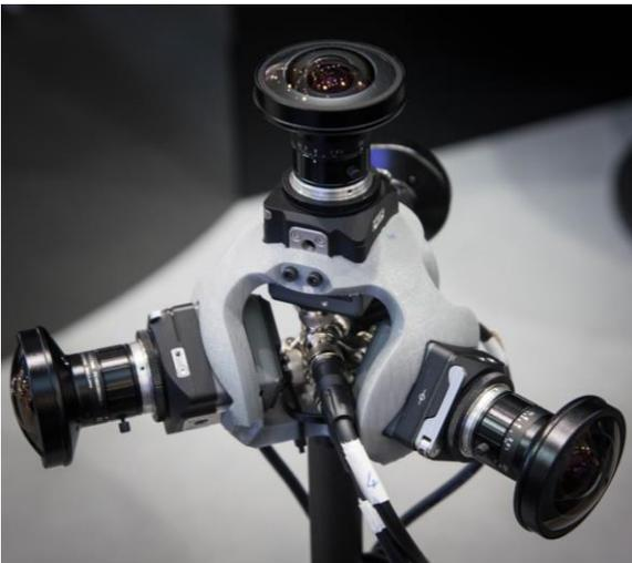
The tiny HD Professional camera SinaCam in this device is able to fully show her well known, unique features, which are popular among filmmakers: The 2/3" CCD sensor, the large dynamics width (13.5f-stops), the 14-bit image processing, up to 60 fps frame rate and the simple
